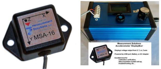
The MSA is a small, low power, complete 3-axis accelerometer with signal conditioned analog voltage outputs. It can measure the static acceleration of gravity in Tilt & Angle applications, as well as dynamic acceleration resulting from motion, shock, or vibration.
